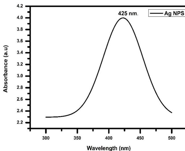
Fig. 1b. UV- Vis spectra of synthesized Silver nanoparticles of *D. carota*
