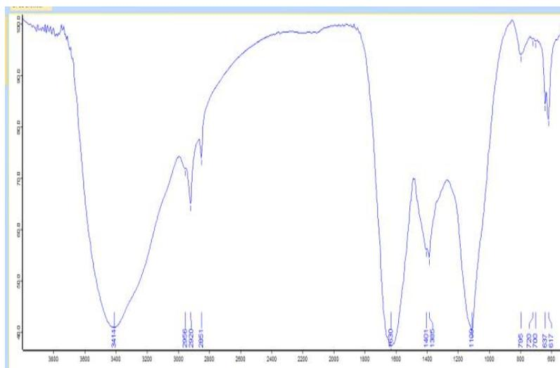
Fig. 4d. Fourier Transformed Infrared Spectroscopy of AgNPs from *Daucus carota*
